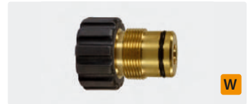
M27 AG : 3/8" IG. Messing *. Max. 400 bar
