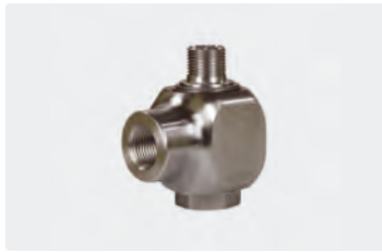
3/8" IG : 3/8" AG. DN 10. Max. 30 U/min / 90 °C
